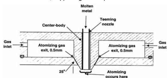
Figure 4. Schematic view of atomizing nozzle and plenum chamber.
