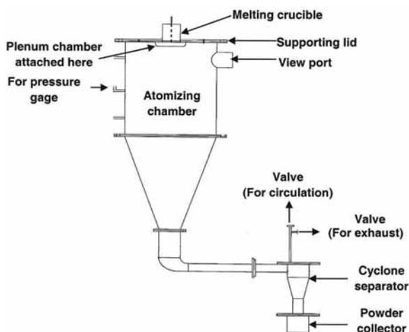
Figure 2. Schematic view of Indigenous Gas Atomizer.
