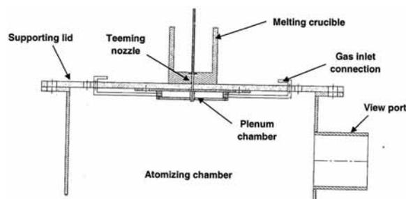
Figure 3. Schematic view of assembly consisting of melting crucible, supporting lid and plenum chamber.
