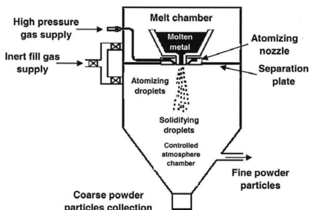
Figure 1. Schematic view of a typical Gas Atomizer [6].
