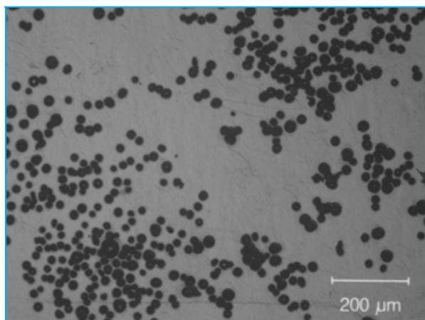
Figure 6b. Optical micrograph of Cu powder particles produced at 10 bar of atomizing gas pressure.
