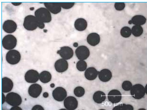
Figure 6a. Optical micrograph of Cu powder particles produced at 2 bar of atomizing gas pressure.
