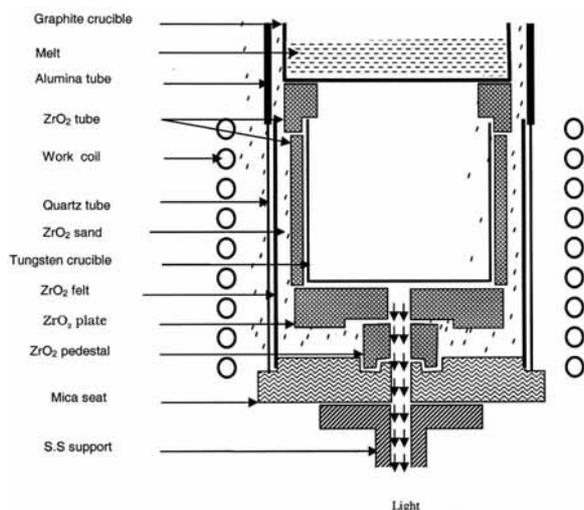
Figure 1. Schematic diagram of crystal growth station for Ge crystals
