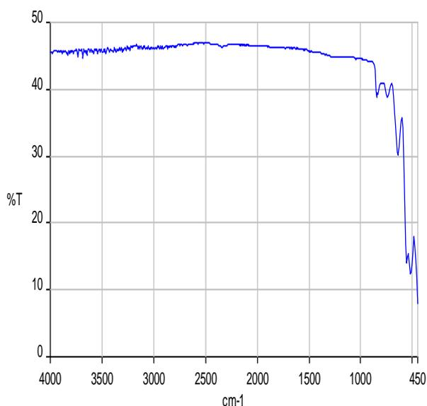
Figure 6. IR Transmission of grown Ge crystal (uncoated). Thickness = 3mm.
