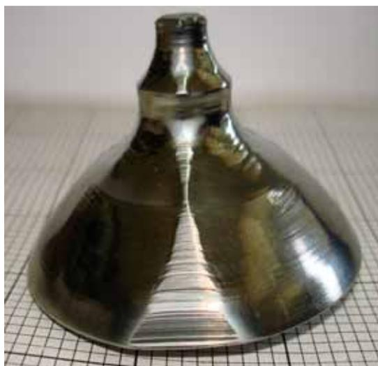
Figure 3. Typical grown Ge single crystal.
