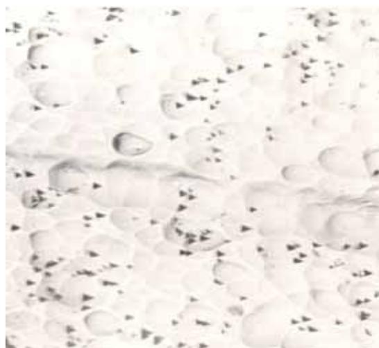
Figure 5. Etch-pits on (111) surface, Magnification 80X.
