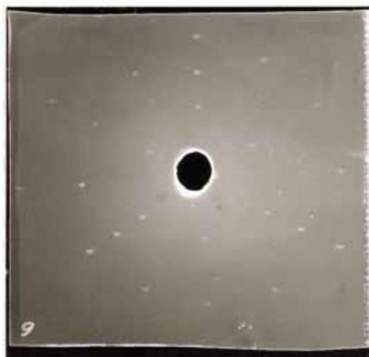
Figure 4. Back reflection of X-rays Laue picture of (111) surface.
