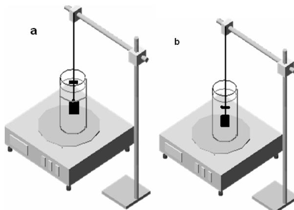
Figure 2. Setup of proposed 'Alternate' method on toploading balance, for density measurements of solid objects lighter than water. (a) only heavy object is dipped, (b) both heavy and lighter objects are dipped.
