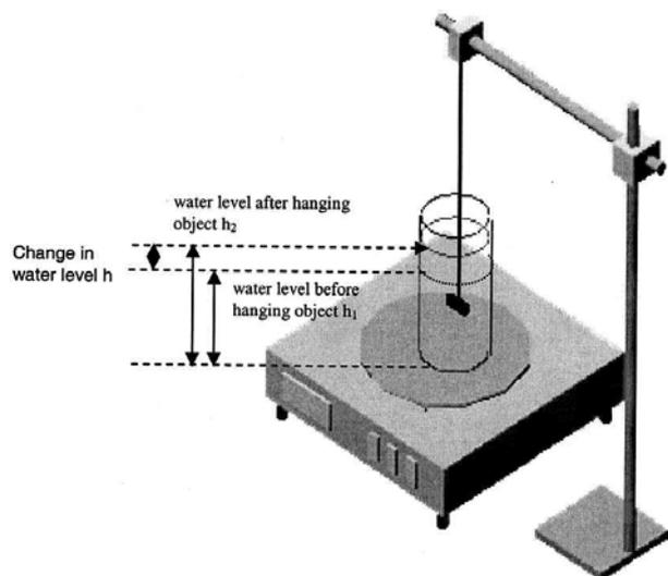
Figure 1. Setup of proposed 'Alternate' method on toploading balance, for density measurements of solid objects heavier than water.
