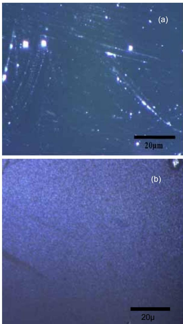
Figure 3. Optical micrograph on same magnification for (a) as grown (b) film annealed at 200 °C.
