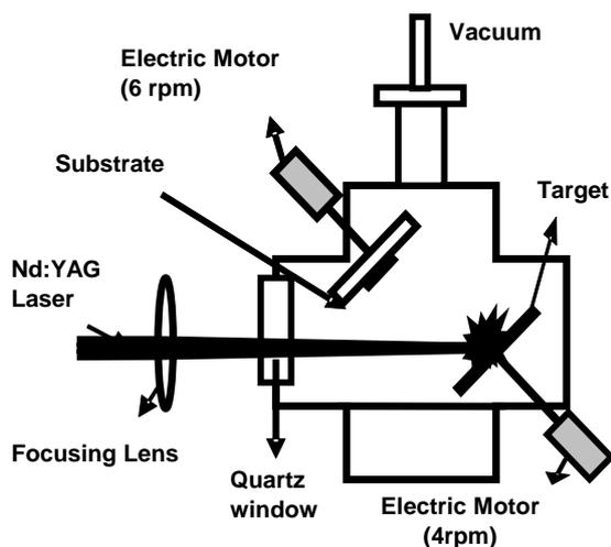
Figure 1. Schematic diagram for the laser ablation system.
