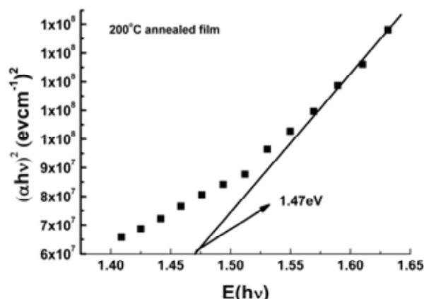
Figure 5. The variation of  $(\alpha h\nu)^2$  with energy ( $h\nu$ ) for the film annealed at 200°C.
