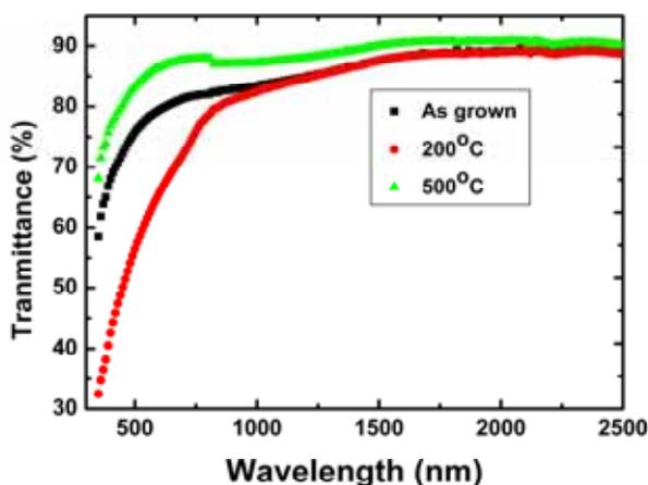
Figure 4. Transmittance versus wavelength for the as grown as well as films annealed at different temperatures.
