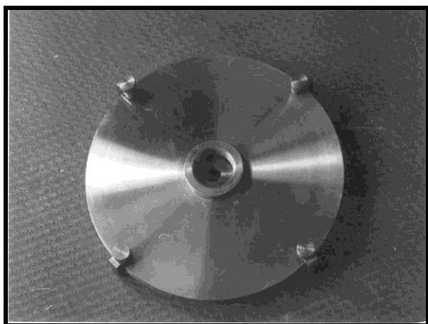
Figure 4. Mould assembly used to fabricate micro-composites with clamping studs in place.
