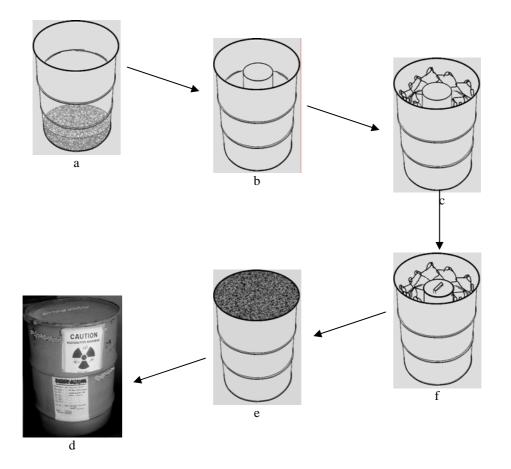
Figure 2. Different steps of DSRS conditioning till the finished package – (a) RCC bottom plug, (b) Inner 4-6 mm MS drum inserted, (c) φ3-4 mm galvanized steel net inserted amid outer and inner drums, (d) DSRS package inserted and covered into inner drum, (e) Concrete poured into the assembly with on-top RCC plug, (f) Finished package with engraved as well as painted markings ready for Interim storage.
