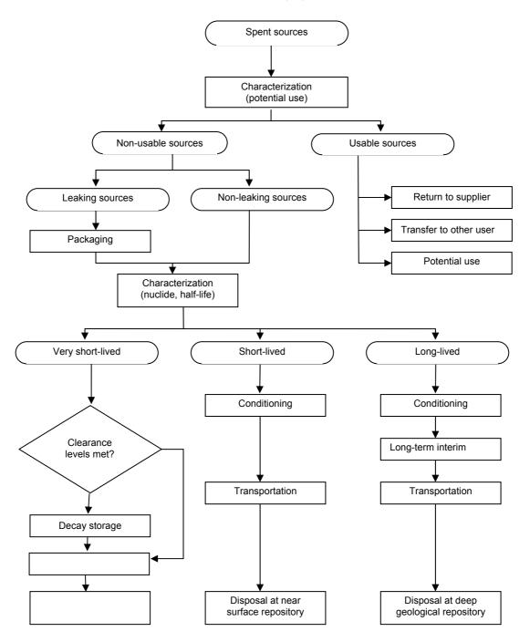
Figure 1. Schematic diagram of SRS management proposed by IAEA [16].
