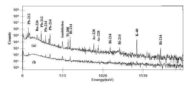
Figure 2. Comparison of gamma spectra: (a) Sediment sample (b) Background of the system.
