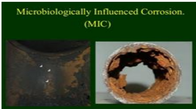
Fig. 2: Microbiologically induced corrosion on a metal surface [6]
