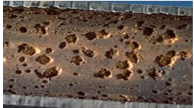
Fig. 3: Pitting corrosion on steel [6]
