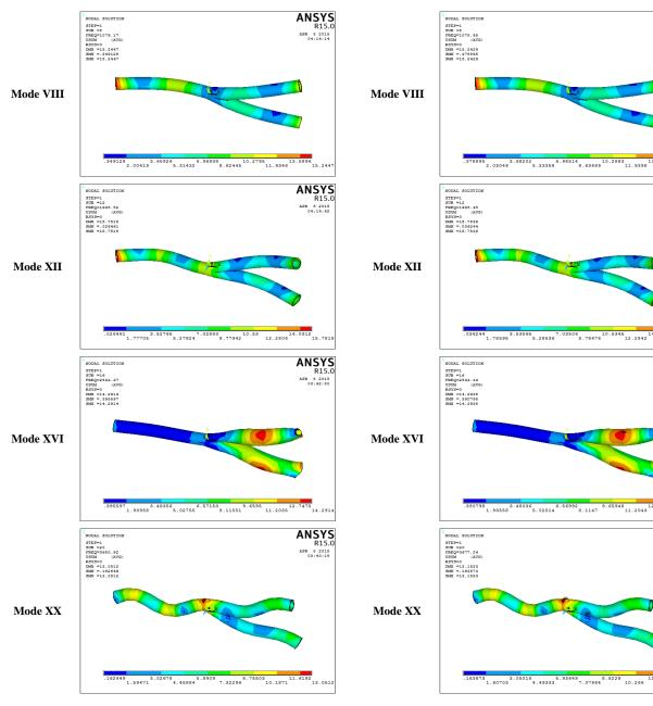
Figure 5d: Mode Shapes for Case-1 with crack depth (a/d=0.6)
