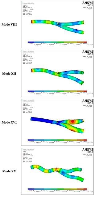
Figure 5c: Mode Shapes for Case-1 with crack depth (a/d=0.4)
