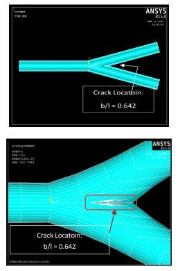
Figure 4: Crack modeling in ansys
