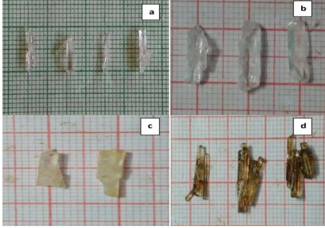
Fig. 1: As grown (a) pure LTMA (b) Zn 2+ doped LTMA (c) Cd 2+ doped LTMA (d) Pb 2+ doped LTMA single crystals
