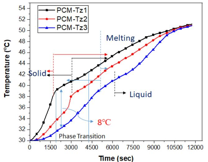
Fig. 5: Temperature profile of pure paraffin along z-axis
