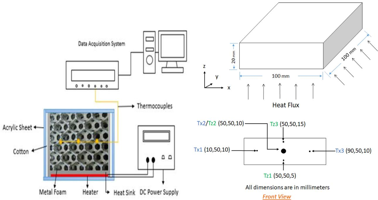
Fig. 2: Schematic view of the experimental setup and thermocouple positioning.
