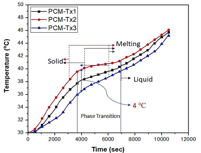
Fig. 4: Temperature profile of pure paraffin along x-axis
