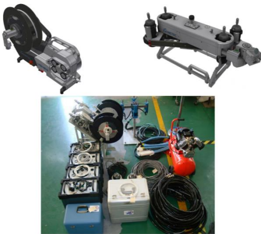
Fig. 9: Typical ET SG Tubes Inspection System
