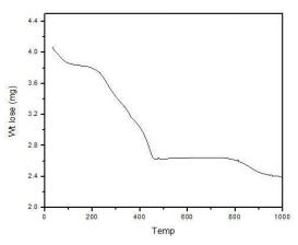
Fig. 4: TGA analysis of synthesized silver nanoparticles by using leaves extract of *S. cumini*
