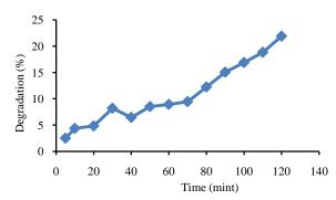
Fig. 7: % degradation of MO dye of synthesized silver nanoparticles
