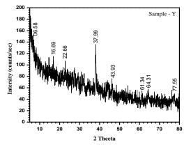
Fig. 2: XRD analysis of synthesized silver nanoparticles by using leaves extract of *S. cumini*
