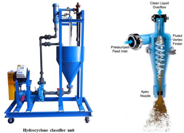
Fig. 3: Hydrocyclone classifier (laboratory scale) with overflow and underflow fractions.
