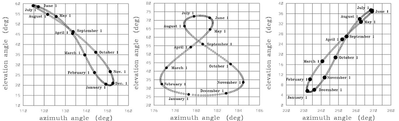
Fig. 11 Analemma for the year 2013. The observer is located at a latitude  $\delta=40.73^\circ$ . The solar azimuth angle measured from north  $\alpha_a$  (degrees), see Eq. (14), as the abscissa and the solar elevation angle  $\alpha_e$  (degrees), see Eq. (7), as the ordinate. Left panel: Analemma at 10:00 A.M. Middle panel: Analemma at noon. Right panel: Analemma at 4:00 P.M.
