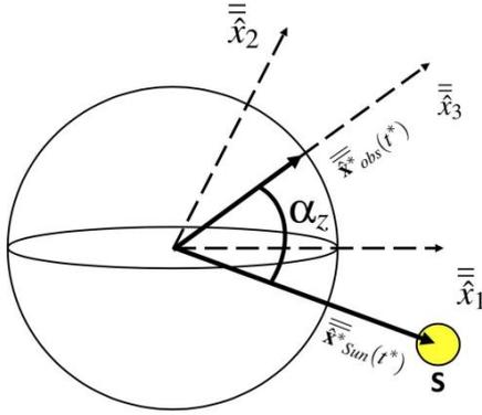
Fig. 4 The observer position vector  $\bar{\hat{x}}_{obs}^*(t^*)$ , the Sun position vector  $\bar{\hat{x}}_{Sun}^*(t^*)$  and the solar zenith angle  $\alpha_z$  in the Cartesian coordinate system  $o, \bar{\hat{x}}_1, \bar{\hat{x}}_2, \bar{\hat{x}}_3$ .
