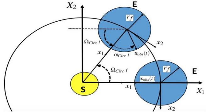
Fig. 8 Circular trajectory of the fictitious Earth: the moving coordinate system  $(o, x_1, x_2)$ , rotates by an angle  $\Omega_{\text{Circ}} t$ . In the moving coordinate system, the position of an observer on the fictitious Earth surface is given as  $x_{\text{obs}}(t) = r_f \cos((\omega_{\text{Circ}} + \Omega_{\text{Circ}})t) i_1 + r_f \sin((\omega_{\text{Circ}} + \Omega_{\text{Circ}})t) i_2$ , where  $r_f$  is the unit radius of the fictitious Earth.
