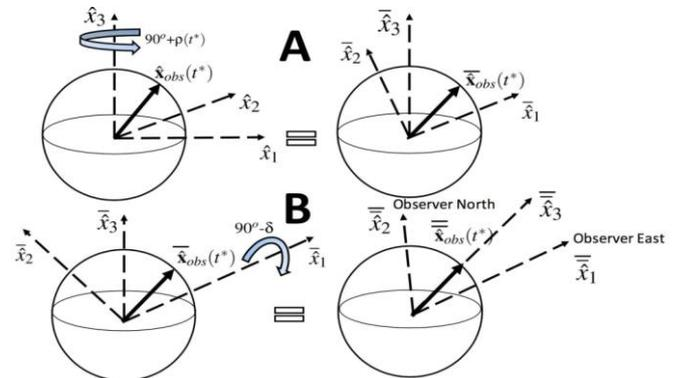
Fig. 3 Transformation matrices A and B from the Cartesian coordinate system  $o, \hat{x}_1, \hat{x}_2, \hat{x}_3$  to the Cartesian coordinate system  $o, \bar{\hat{x}}_1, \bar{\hat{x}}_2, \bar{\hat{x}}_3$ .
