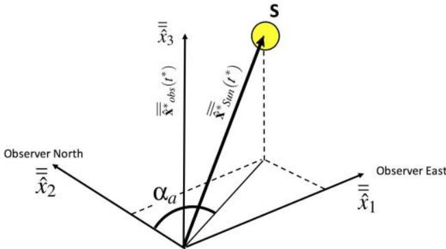
Fig. 5 The observer position vector  $\bar{\hat{x}}_{obs}^*(t^*)$ , the Sun position vector  $\bar{\hat{x}}_{Sun}^*(t^*)$  and the solar azimuth angle measured from north  $\alpha_a$  in the Cartesian coordinate system  $o, \bar{\hat{x}}_1, \bar{\hat{x}}_2, \bar{\hat{x}}_3$ . The observer horizon plane is defined by the plane  $\bar{\hat{x}}_1 - \bar{\hat{x}}_2$ , where  $\bar{\hat{x}}_1$  is the observer's East while  $\bar{\hat{x}}_2$  is the observer North.
