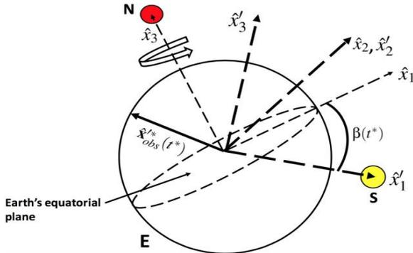
Fig. 1 Cartesian coordinate system  $(o, \hat{x}'_1, \hat{x}'_2, \hat{x}'_3)$ , whose origin is located at the center of the Earth. Its axis  $\hat{x}'_1$  always points towards the Sun. Its axis  $\hat{x}'_2$  always coincides with the axis  $\hat{x}_2$  of the fixed Cartesian coordinate system  $o, \hat{x}$ . It oscillates, from  $\beta(t^*) = -23.45^\circ$  to  $\beta(t^*) = +23.45^\circ$ , about its axis  $\hat{x}'_2$ .
