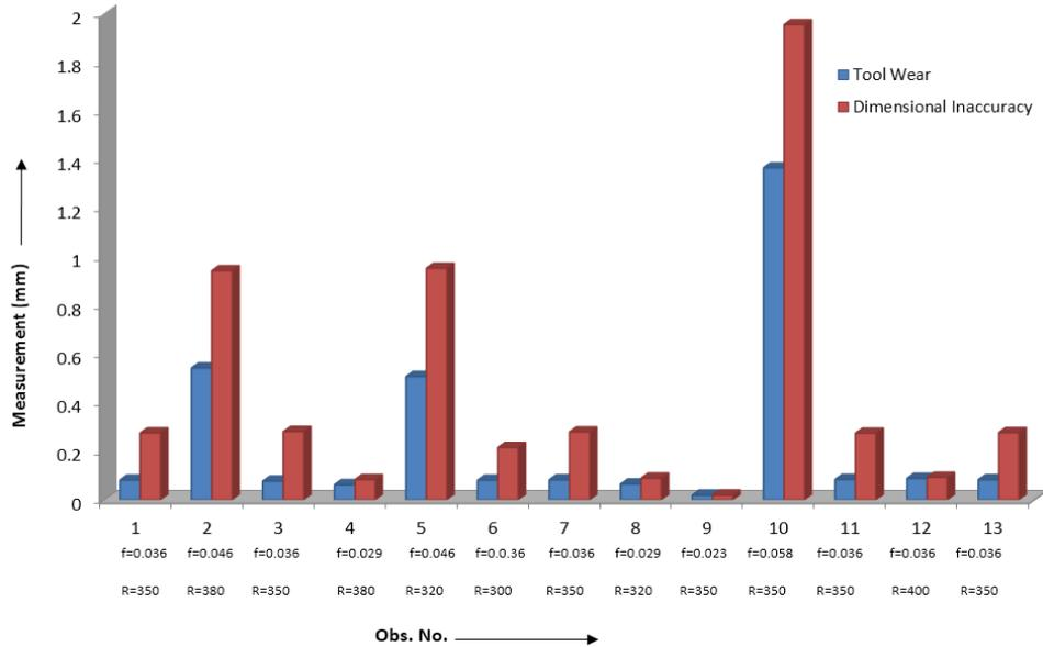
Fig. 5: Radial tool wear and dimensional inaccuracy for workpiece-arc with 1.5mm radius.
