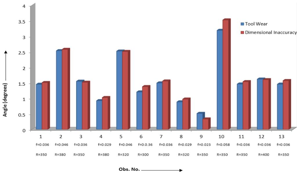
Fig. 4: Angular variation of tool wear and dimensional inaccuracy for form tool- angle of 54°
