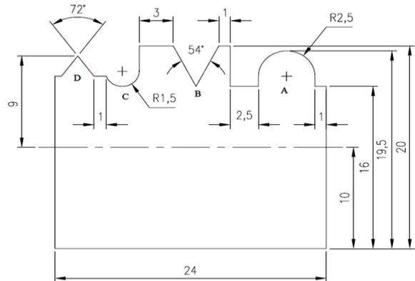
A. Interior arc with 2.5mm radius      B. Triangle with included angle of 54°
