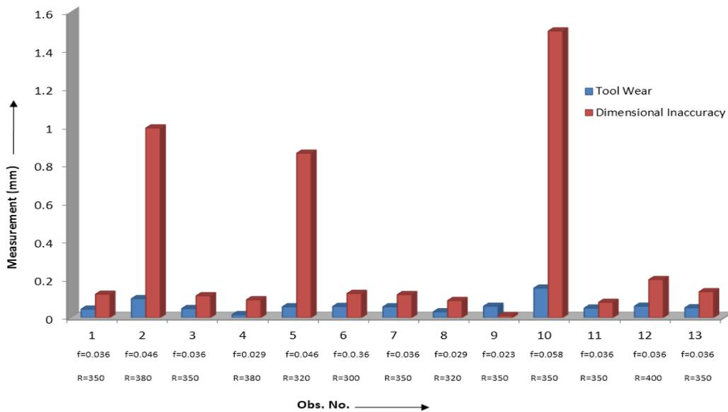
Fig. 3: Radial tool wear and dimensional inaccuracy for form tool-internal arc of 2.5mm radius
