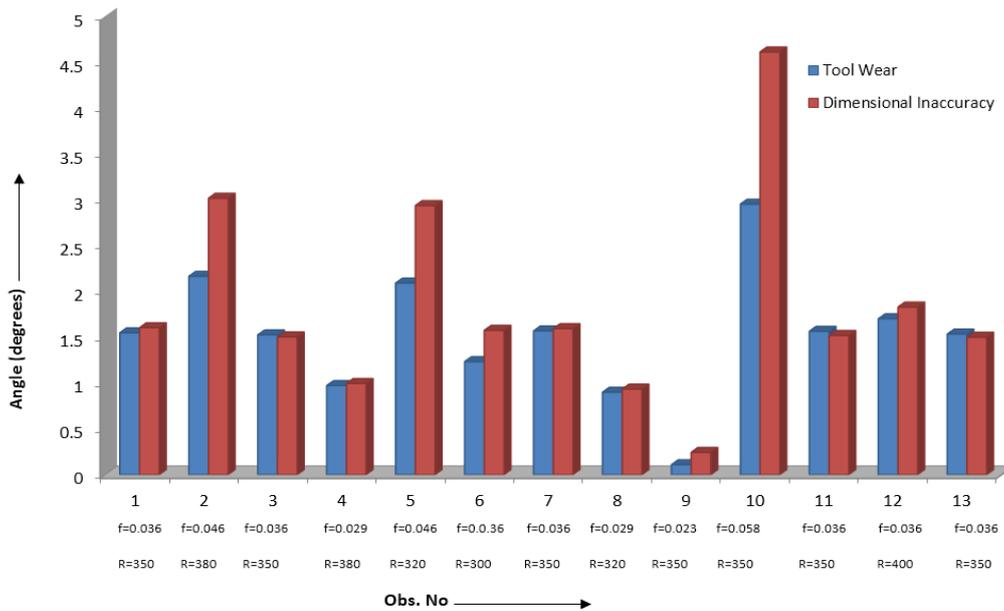
Fig. 6: Angular tool wear and dimensional inaccuracy for workpiece-Angle of 72°
