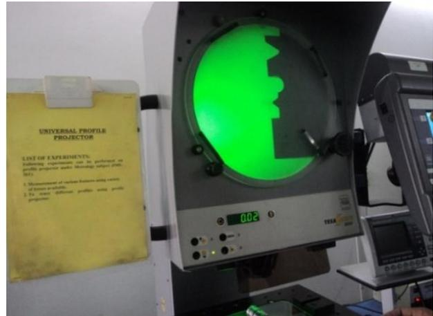
Fig. 2: Measurement of work-piece profile after the turning operation using Universal Profile Projector
