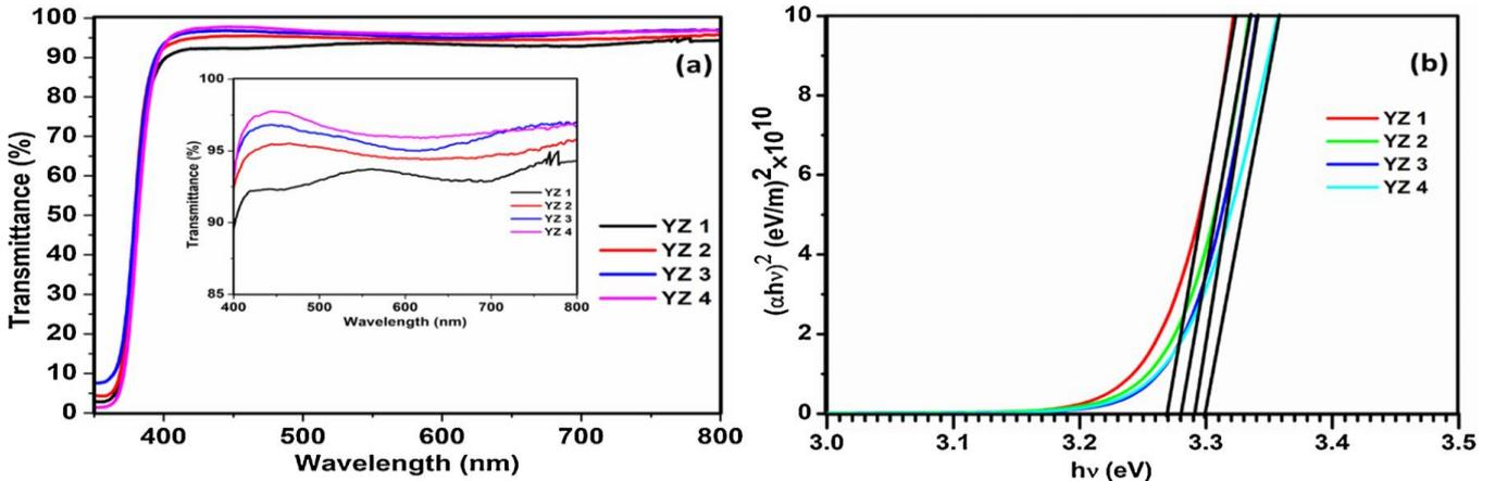
Figure 4: Optical properties of ZnO thin-film doped with Y: Transmission (a) and optical band gap (b)
