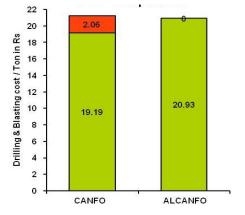
Fig. 8: Economics of conventional and modified blast at bench # 3
