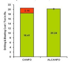
Fig. 7: Economics of conventional and modified blast at bench # 2
