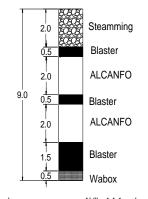
Fig. 3: Charging sequence, modified blasting at bench # 2
