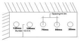
Fig. 4: Firing pattern of holes at bench # 3
