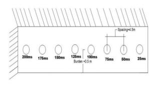
Fig. 1: Firing pattern of conventional & modified blasts at bench # 2
