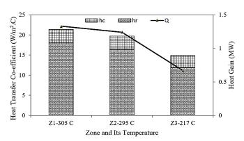
Fig. 5: Effect of temperature on coefficient of radiation and convection.
