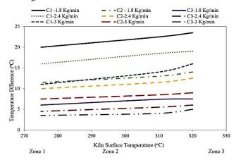
Fig. 9: Effect of kiln surface temperature on temperature difference at (a) 1.8 kg/min (b) 2.4 kg/min (c) 3 kg/min.
