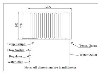
Fig. 2: Schematic of heat recovery system.
