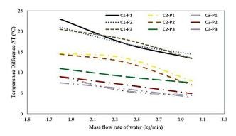
Fig. 8: Effect of mass flow rate of water on temperature difference at positions 1, 2 and 3 on corresponding radial distances.
