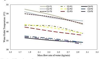
Fig. 7: Effect of mass flow rate of water on heat water outlet temperature at heat recovery device at positions 1, 2 and 3 on corresponding radial distances.
