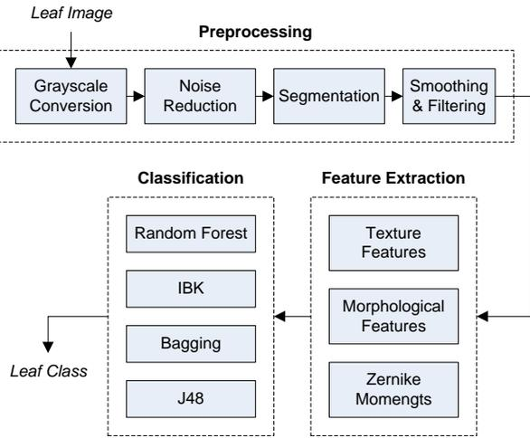
Fig. 2: Detailed working of proposed approach.
