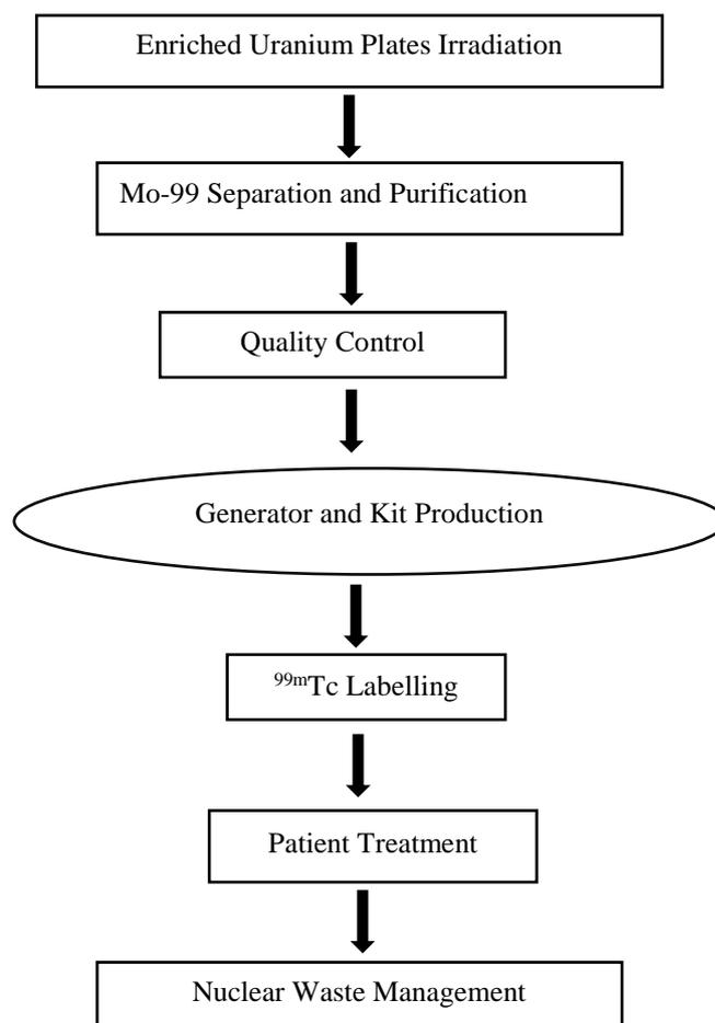
Fig. 1: Life-cycle of <sup>99m</sup>Tc radioisotope.
