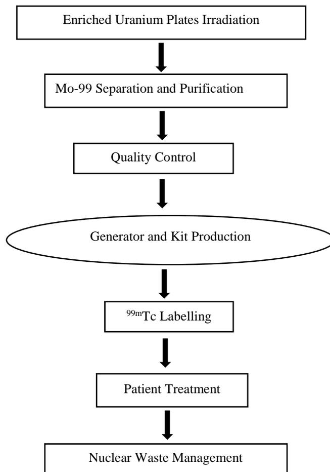
Fig. 1: Life-cycle of <sup>99m</sup>Tc radioisotope.
