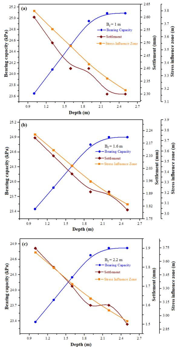
Fig. 8: Effect of strip footing on bearing capacity, settlement and stress influence zone keeping width fixed and varying depth (a)  $b_f = 1\text{ m}$  (b)  $b_f = 1.6\text{ m}$  (c)  $b_f = 2.2\text{ m}$ .
