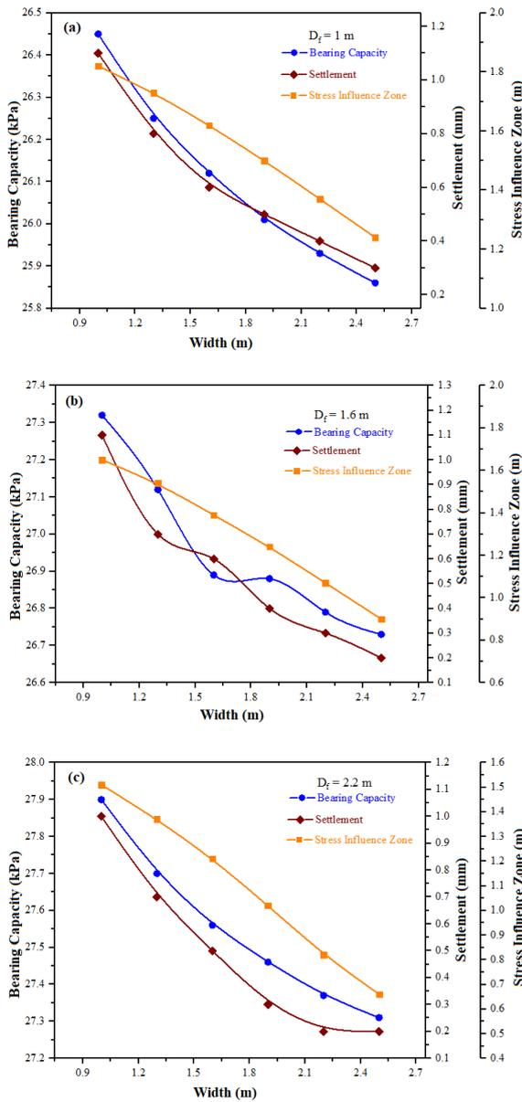
Fig. 3: Effect of square footing on bearing capacity, settlement and stress influence zone keeping depth fixed and varying width (a)  $d_f = 1\text{ m}$  (b)  $d_f = 1.6\text{ m}$  (c)  $d_f = 2.2\text{ m}$ .
