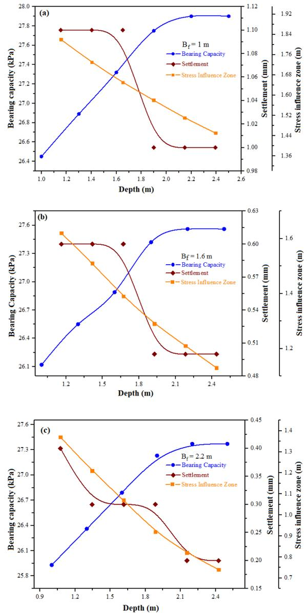
Fig. 4: Effect of square footing on bearing capacity, settlement and stress influence zone keeping width fixed and varying depth (a)  $b_f = 1\text{ m}$  (b)  $b_f = 1.6\text{ m}$  (c)  $b_f = 2.2\text{ m}$ .
