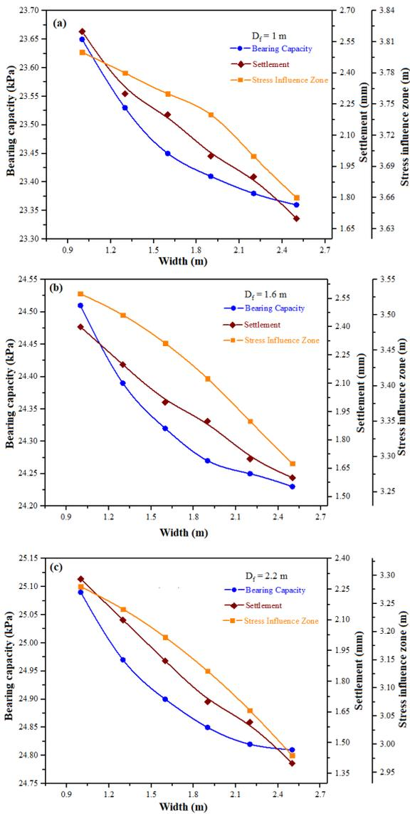
Fig. 7: Effect of strip footing on bearing capacity, settlement and stress influence zone keeping depth fixed and varying width (a)  $d_f = 1\text{ m}$  (b)  $d_f = 1.6\text{ m}$  (c)  $d_f = 2.2\text{ m}$
