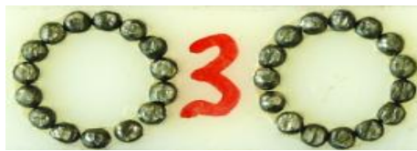
Fig. 3: Un-deformed specimen filled with lead balls
