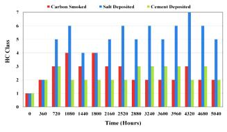
Fig. 4. Hydrophobicity classification of all samples.
