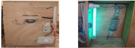
Fig. 1. Photographs of a multi stress aging chamber, outside (left) and inside (right).
