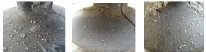
Fig. 3. Hydrophobicity of samples after 5040 hours of aging carbon smoked (left), cement deposited (center), salt deposited (right).
