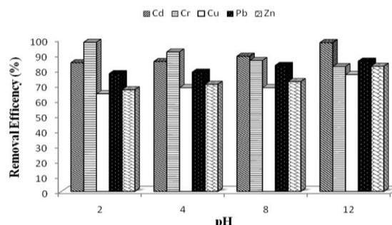
Figure 2. Removal efficiency of paper mulberry bio-char at different pH.
