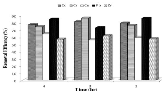
Figure 4. Removal efficiency of paper mulberry bio-char at different contact time.
