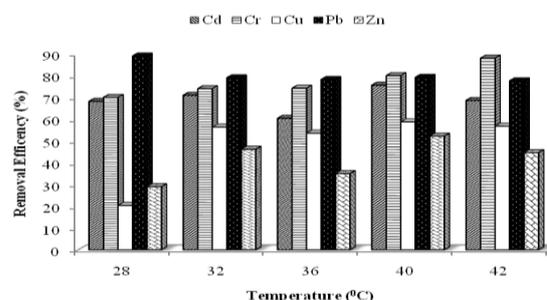
Figure 3. Removal efficiency of paper mulberry bio-char at different temperatures.
