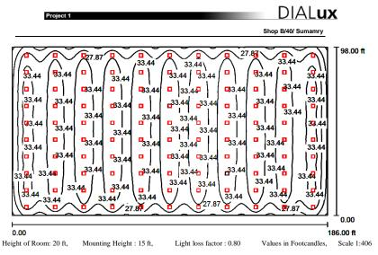
Figure 3. Lay out design of B-40 shop by using DIALux 4.11.
