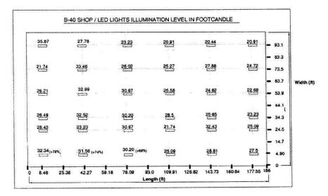
Figure 5. B-40 shop / LED lights illumination level in foot candle.
