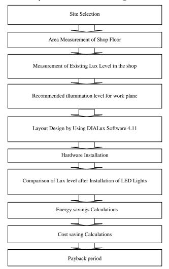
Figure 1. Flow chart for an energy conservation scheme.
