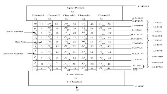
Figure 1. Schematic diagram of the model prepared for EUREKA-2/RR analysis.
