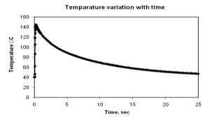
Figure 4. Temperature change with time in fresh core.
