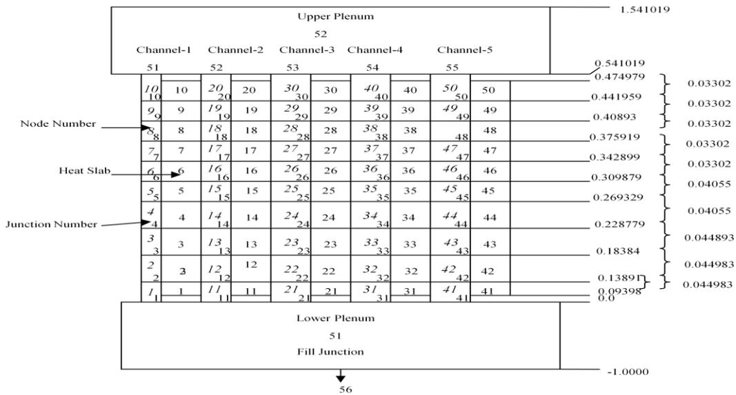
Figure 1. Schematic diagram of the model prepared for EUREKA-2/RR analysis.
