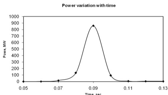
Figure 3. Power change with time in fresh core.
