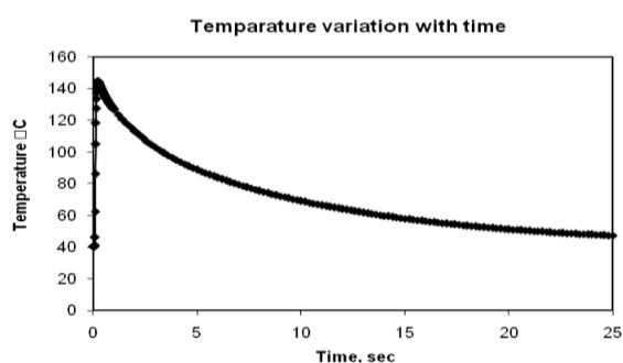
Figure 4. Temperature change with time in fresh core.
