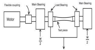
Figure 3. Fatigue test experimental setup.
