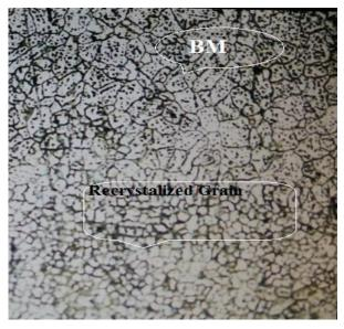
Figure 8. Recrystallization of grains in II pass of welding.
