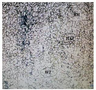
Figure 7. Grain structure of different zones
