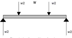
Figure 4. Loading conditions of specimen.
