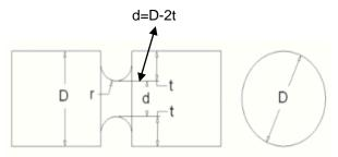
Figure 5. Notch specification of specimen.
