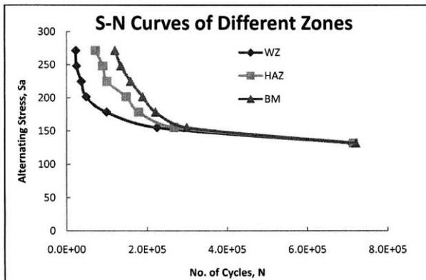
Figure 6. S-N Curves of different welding zones.
