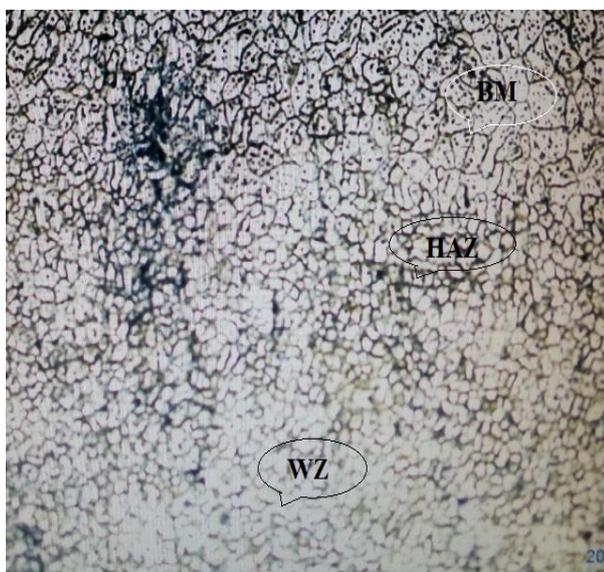
Figure 7. Grain structure of different zones
