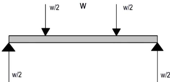
Figure 4. Loading conditions of specimen.
