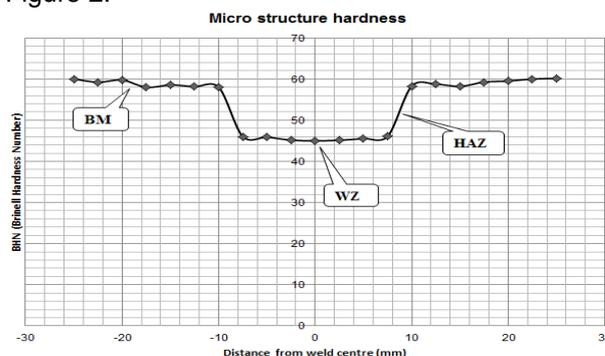
Figure 2. BHN of different welding zones.
