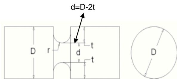
Figure 5. Notch specification of specimen.
