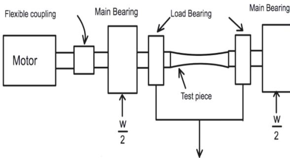
Figure 3. Fatigue test experimental setup.
