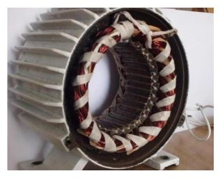
Figure 4. Stator of generator model.
