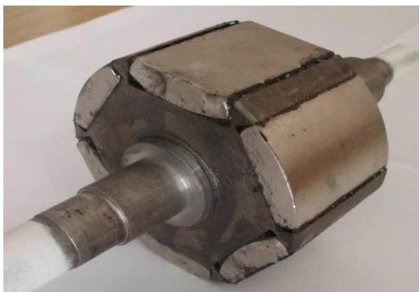
Figure 7. Rotor of generator model with magnets.
