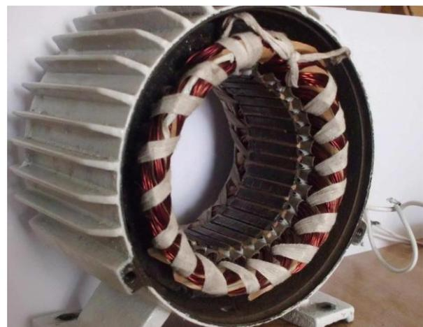
Figure 4. Stator of generator model.
