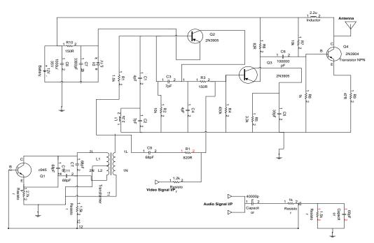
Figure 3. The schematic diagram of TV transmitter.
