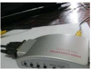
Figure 7a. VGA Converter.
