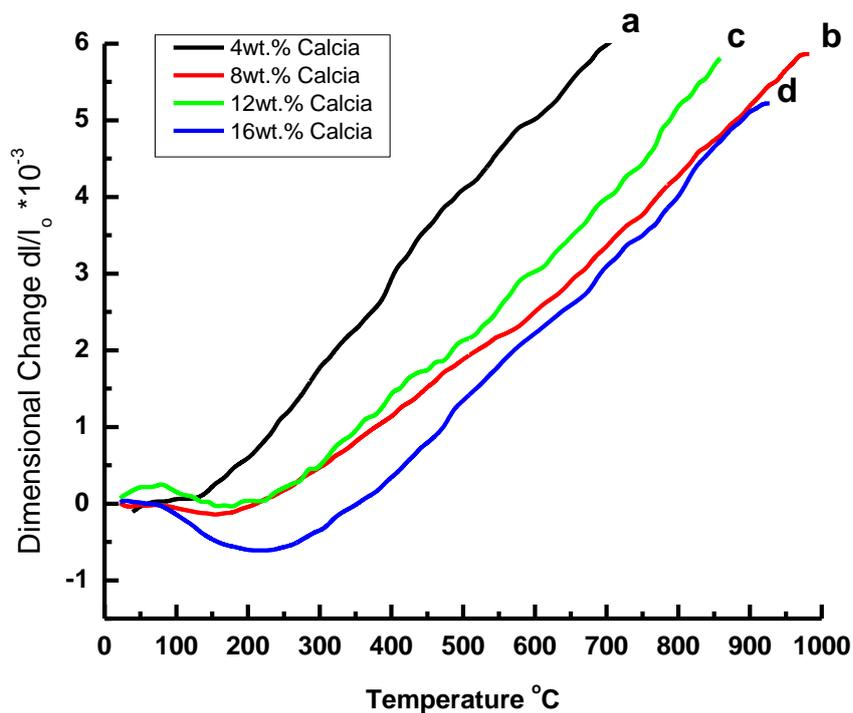
Figure 3 (a-c). Dilatometric curves of calcia stabilized zirconia (a) 4CSZ (b) 8CSZ (c) 12CSZ and (d) 16CSZ.
