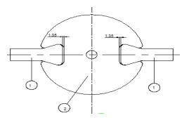
Figure 5. Assembly of two sectors of disc and blades in dovetail joints.
