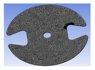
Figure 13. The model of disc after meshing
