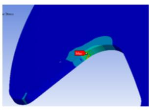
Figure 16. Maximum shear stress at stress probe 4. Table 3. Stress variation at stress P**r**obes 1~7.
