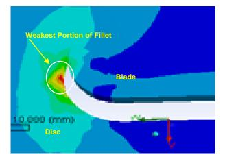
Figure 20. Maximum principal stress at stress probe 4 (crack initiation tip).
