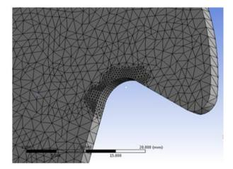
Figure 14. The enlarged view of model of disc after meshing in critical region.
