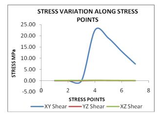
Figure 17. Trend of shear stress variation at stress probes  $1 \sim 7$ .
