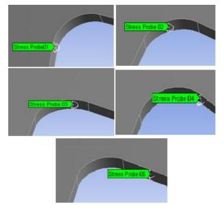
Figure 15. The stress probe 1.2,3,4 and 5 on the fillet surface of the disc.
