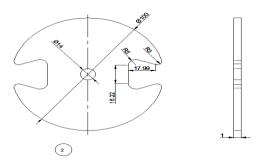
Figure 6. Drawing and dimensions of the disc.
