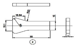
Figure 7. Drawing and dimensions of blades.
