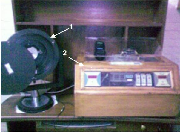
Figure 1. Experimental testing rig showing (1) the assembly testing fixture and (2) speed control system of the rig.
