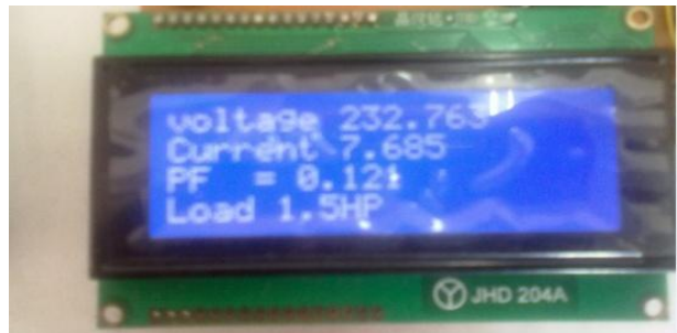
Figure 28. Load monitoring for 1.5hp inductive load.
