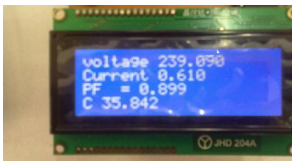
Figure 18. LCD showing selected value of 'C' for desired PFC.
