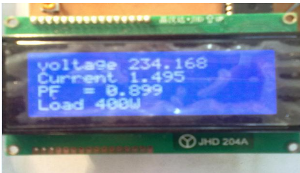
Figure 14. Load monitoring for resistive load.
