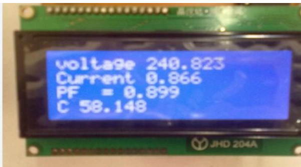
Figure 24. LCD showing selected value of 'C' for desired PFC.
