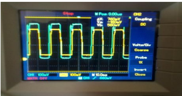
Figure 31. Zero crossing detection after correction with 1.5hp inductive load.
