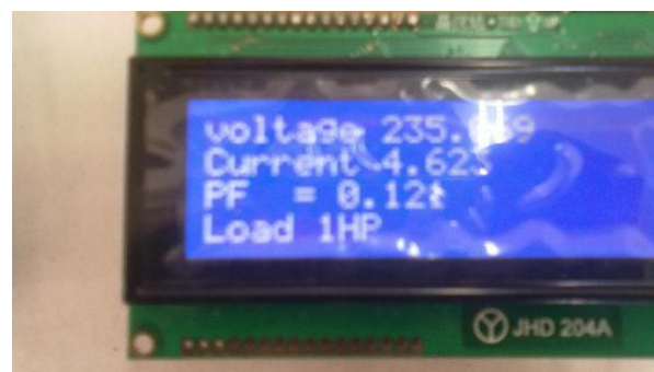
Figure 23. Load monitoring for 1hp inductive load.
