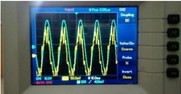
Figure 30. V and I behavior after correction with 1.5hp inductive load.
