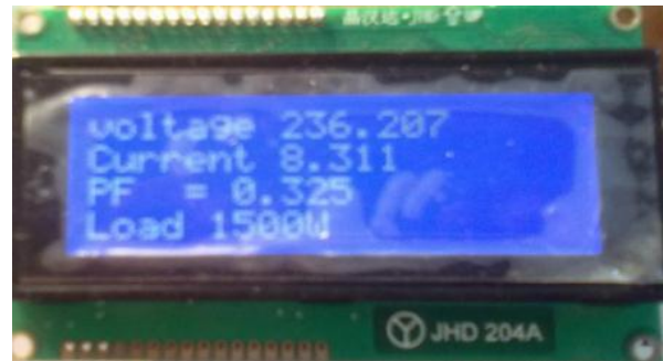
Figure 33. Load monitoring for resistive and inductive load.
