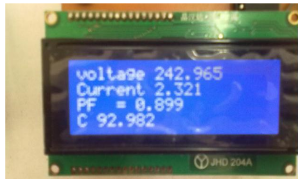
Figure 35. LCD showing selected value of 'C' for desired PFC.
