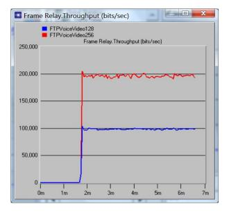
Figure 11. Throughput results for the FTP, Voice & Video applications executing simultaneously on workstations.
