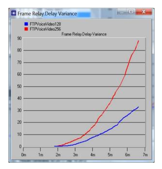
Figure 13. Delay variance for simultaneous execution of FTP, Voice and Video application.
