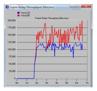
Figure 5. Throughput results for the Voice application executing on workstations.
