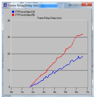
Figure 12. Delay incurred for simultaneous execution of FTP, Voice and Video application.
