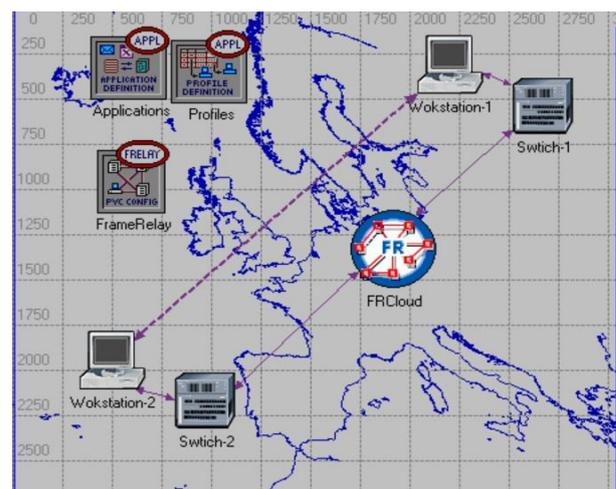
Figure 1. The main scenario describing and Frame Relay based network with 2 workstations communicating with each other through switches connected to a Frame Relay cloud. A PVC is maintained between the workstations for efficient transmission of data.
