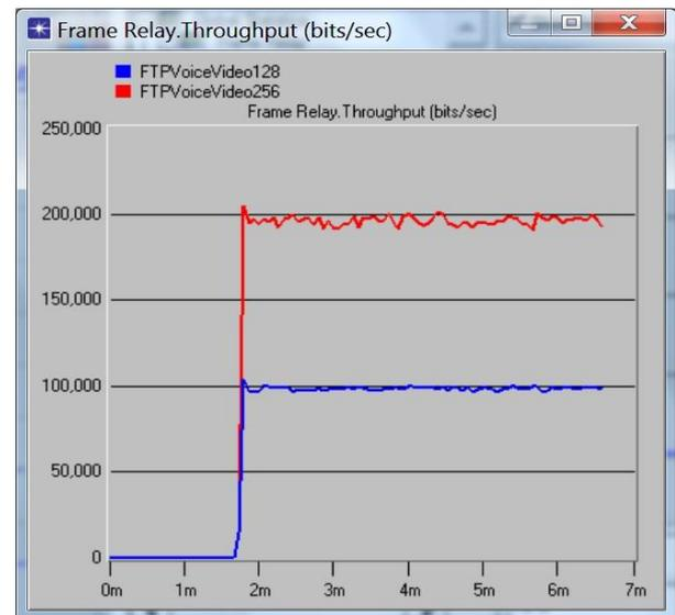
Figure 11. Throughput results for the FTP, Voice & Video applications executing simultaneously on workstations.
