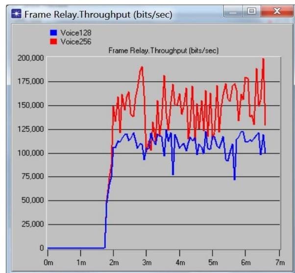
Figure 5. Throughput results for the Voice application executing on workstations.
