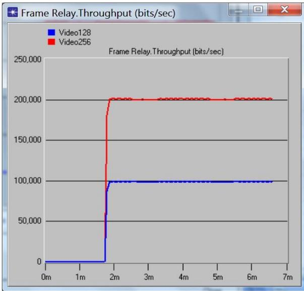
Figure 8. Throughput results for the Video application executing on workstations.
