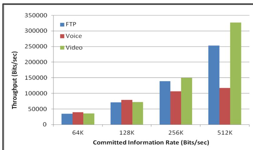
Figure 14. Throughput corresponding to different values of CIR parameter (64K, 128K, 256K, 512K) and BC=128K, BE=32K.
