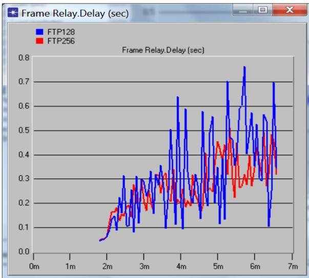
Figure 3. Delay incurred for the FTP application
