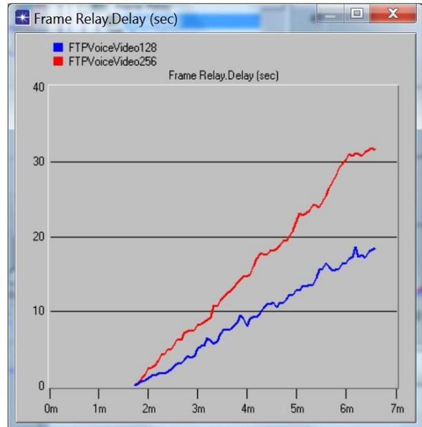
Figure 12. Delay incurred for simultaneous execution of FTP, Voice and Video application.
