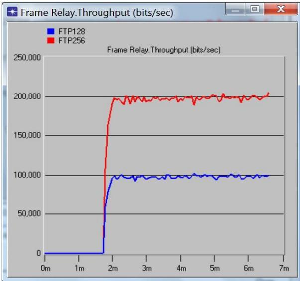
Figure 2. Throughput results for the FTP application executing on workstations
