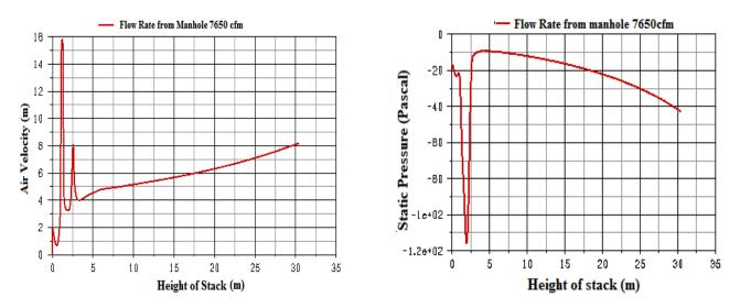
Figure 6a. Air velocity (m/sec) profile at air flow rate (cfm) of 7650 cfm from manhole; (b) Static pressure (Pa) profile at air flow rate (cfm) of 7650 cfm from manhole.
