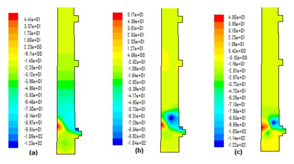
Figure 4. Static pressure (Pa) contours showing the impact of different meshing schemes such as (a) Course mesh; (b) Medium mesh; (c) Fine mesh.
