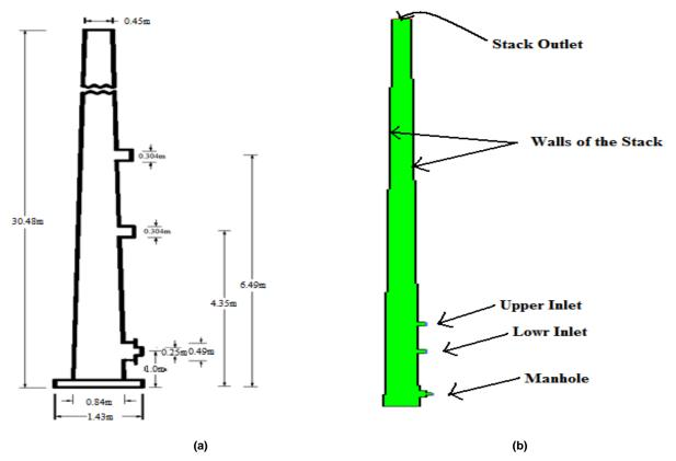
Figure 1. (a) Dimensions of stack (b) Geometry of stack created with GAMBIT.
