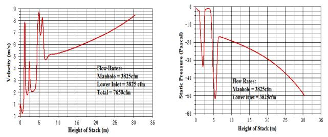
Figure 10. (a) Air velocity (m/sec) profile with 3825 cfm from manhole and lower inlet; (b) Static pressure (Pa) profile with 3825 cfm from manhole and lower inlet.
