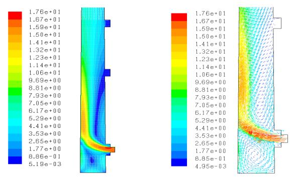
Figure 8a. Velocity contours with air flow rate of 7650 cfm from manhole; (b) Velocity vectors with air flow rate of 7650 cfm from manhole.
