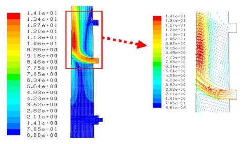
Figure 9. Velocity contours and vectors with air flow rate of 7650 cfm from one of the inlet openings.
