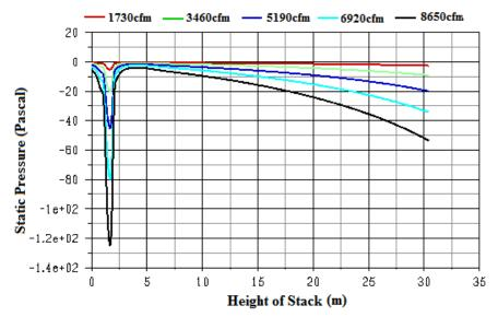
Figure 7. Static pressure (Pascal) profiles with the change in air volumetric flow rate (cfm) from manhole.
