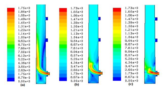
Figure 3. Air velocity (m/sec) contours showing the impact of different meshing schemes such as (a) Course mesh; (b) Medium mesh; (c) Fine mesh.
