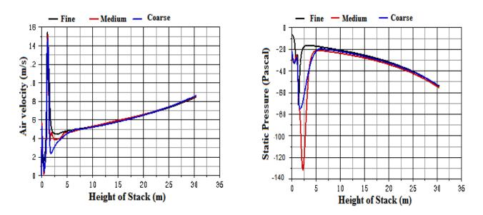
Figure 2. (a) Graph showing the sensitivity of different mesh schemes on air velocity (m/sec); (b) Graph showing the sensitivity of different mesh schemes on static pressure (Pascal).
