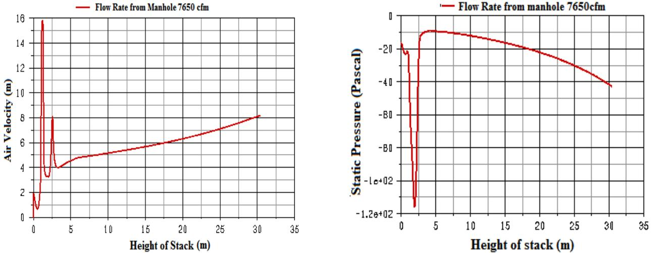
Figure 6a. Air velocity (m/sec) profile at air flow rate (cfm) of 7650 cfm from manhole; (b) Static pressure (Pa) profile at air flow rate (cfm) of 7650 cfm from manhole.
