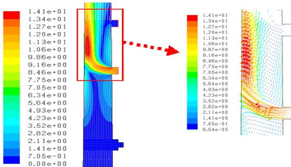
Figure 9. Velocity contours and vectors with air flow rate of 7650 cfm from one of the inlet openings.
