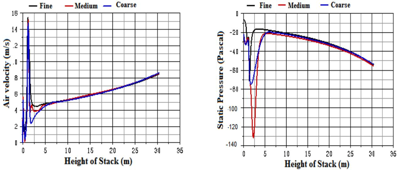
Figure 2. (a) Graph showing the sensitivity of different mesh schemes on air velocity (m/sec); (b) Graph showing the sensitivity of different mesh schemes on static pressure (Pascal).
