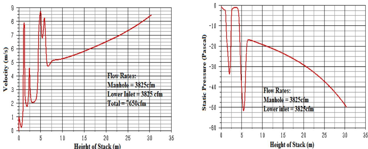
Figure 10. (a) Air velocity (m/sec) profile with 3825 cfm from manhole and lower inlet; (b) Static pressure (Pa) profile with 3825 cfm from manhole and lower inlet.
