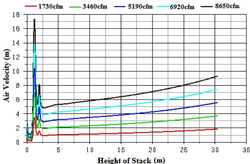
Figure 5. Air velocity (m/sec) profiles with the change in volumetric flow rate (cfm) of air from manhole.
