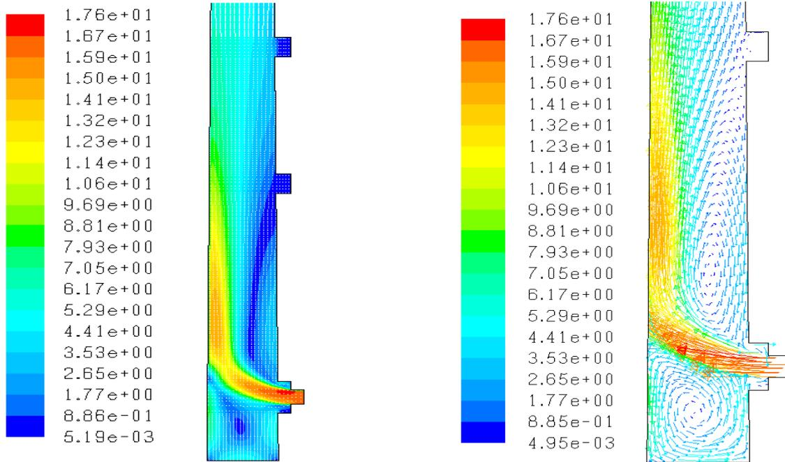
Figure 8a. Velocity contours with air flow rate of 7650 cfm from manhole; (b) Velocity vectors with air flow rate of 7650 cfm from manhole.
