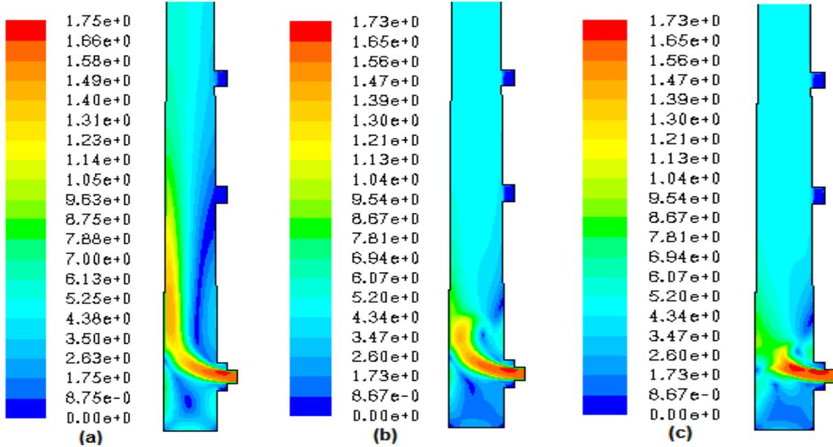
Figure 3. Air velocity (m/sec) contours showing the impact of different meshing schemes such as (a) Coarse mesh; (b) Medium mesh; (c) Fine mesh.
