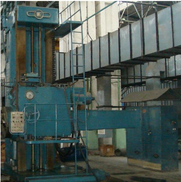
Figure 1. Horizontal boring and milling machine being automated through PLCs.
