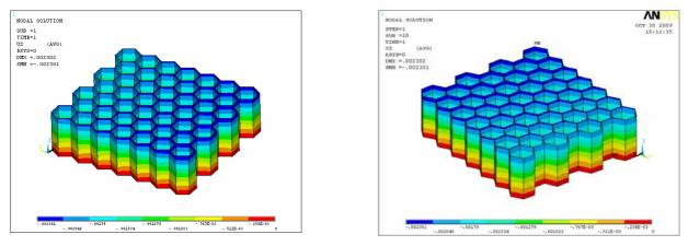
Figure 7. Deformation of FEA model in Z-Directional at the end of Sub-step 1&10
