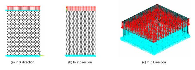
Figure 2. Applied Boundary Conditions for calculation of Ex, Ey and Ez.
