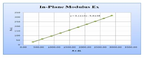
Figure 4. In-Plane Modulus Ex (by FEA).
