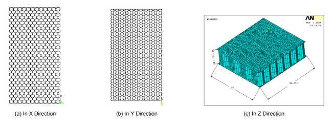
Figure 1. Finite Element Model of the Honeycomb Structure in X, Y and Z Directions
