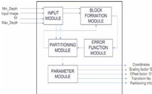
Figure 2. Encoder Block Diagram.
