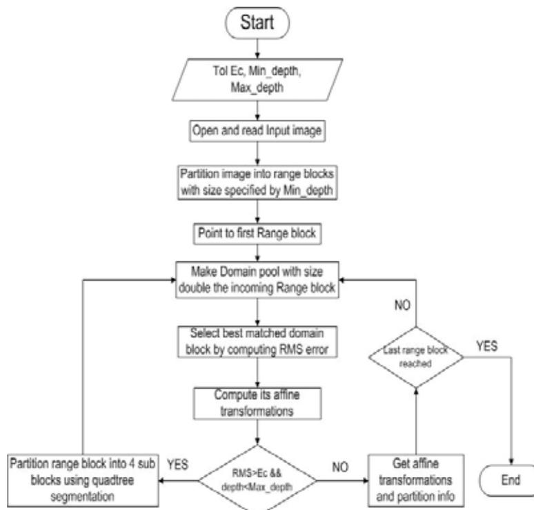
Figure 5. Flowchart for decoding process.
