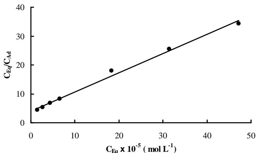
Figure 3. Langmuir adsorption isotherm (Type 1) of silver ions on rice husk.
