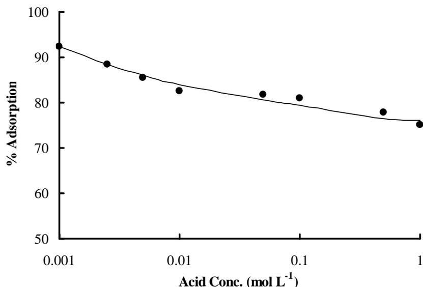
Figure 1. Effect of acid concentration on the percent adsorption of silver ions on rice husk.
