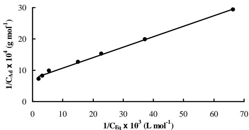
Figure 4. Langmuir adsorption isotherm (Type 2) of silver ions on rice husk.
