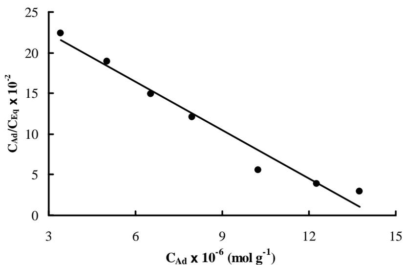
Figure 6. Langmuir adsorption isotherm (Type 4) of silver ions on rice husk.
