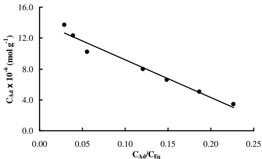
Figure 5. Langmuir adsorption isotherm (Type 3) of silver ions on rice husk.
