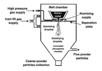
Figure 1. Schematic view of a typical Gas Atomizer [6].
