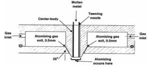
Figure 4. Schematic view of atomizing nozzle and plenum chamber.
