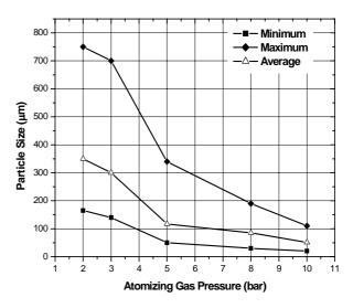
Figure 5. Variation in particles sizes with atomizing gas pressure.
