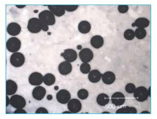
Figure 6a. Optical micrograph of Cu powder particles produced at 2 bar of atomizing gas pressure.
