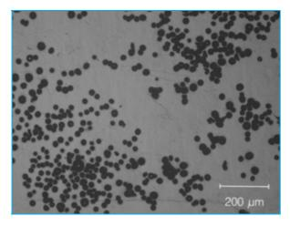
Figure 6b. Optical micrograph of Cu powder particles produced at 10 bar of atomizing gas pressure.
