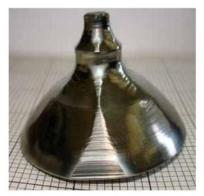
Figure 3. Typical grown Ge single crystal. Max.Dia. =65mm
