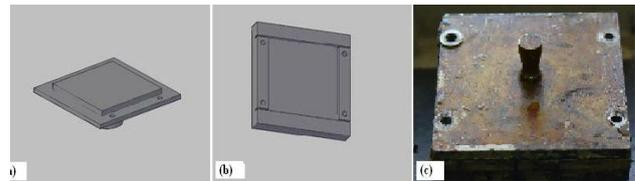
Fig. 1: Schematic of metallic mold (a) Male part, (b) Female part and (c) Picture of the fabricated mold
