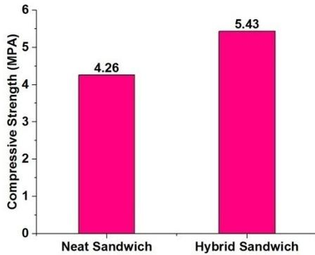
Fig. 4: Compressive strength comparison of neat and hybrid sandwich panel
