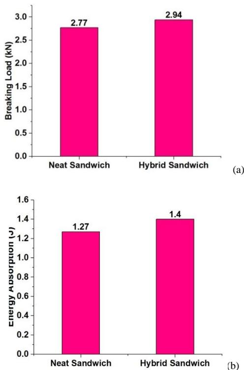
Fig. 7: Quasi-static indentation test results (a) breaking load and (b) energy absorption
