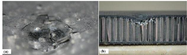
Fig. 8: Photo of indentation damage in sandwich panel after quasi-static indentation test showing (a) fiber breakage and cracking in face sheet and (b) core crushing and local buckling in cross sectional view
