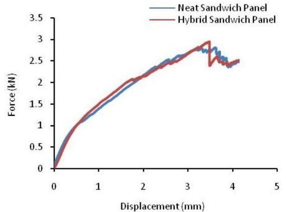
Fig. 6: Force-Displacement curve of both sandwich panels captured during quasi-static indentation test
